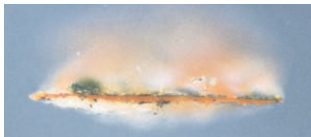
FIG. 10. Madonna and Child with Four Saints (fig. 1), cross-section (200×) from central panel showing the silver ground along the left edge of the mantle below the shoulder; note the restored gold layer directly on top of silver leaf.
